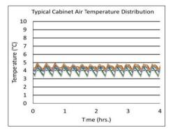
Performance data acquired at 22°C ambient, 4°C nominal set point in an empty cabinet with shelves using air probes, during stabilized steady state operation and a DAQ sampling rate of one measurement every 10 seconds
