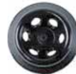
MLXF-7 1.5mL Standard Rotor
