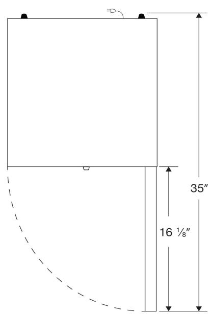
Note: This unit must have 4" clearance on sides and back for adequate ventilation
