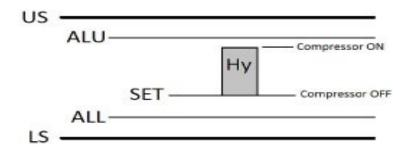
During the normal operation, the refrigerator's (or freezer's) compressor would turn on and off, in order to maintain the cold temperature in the storage chamber.
