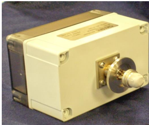
Oxygen monitor with KF flange attached directly to the monitor NOTE: Cell is delicate. When mounted in the corresponding flange it is protected
